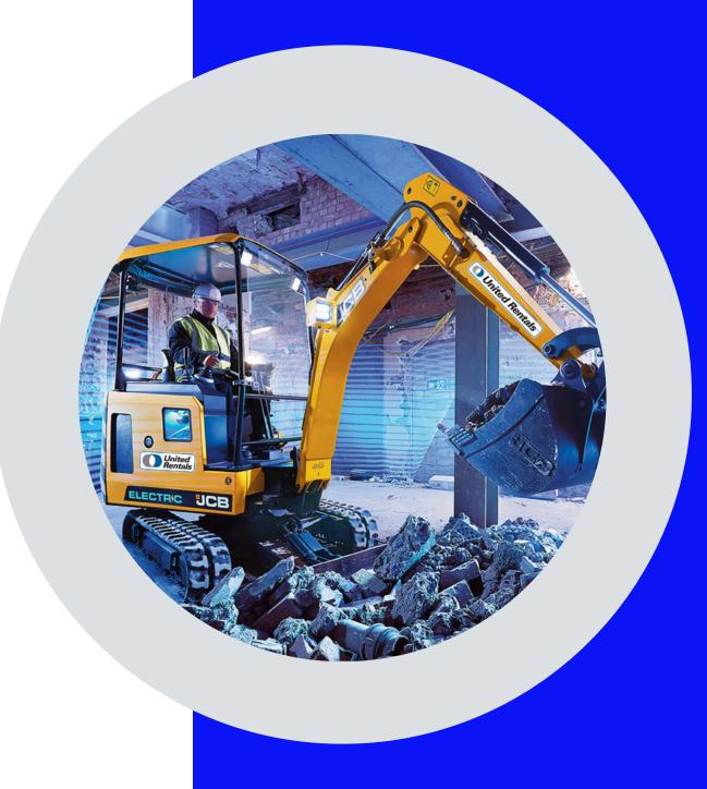
Electric equipment offers performance on par with that of traditionally fueled counterparts while eliminating direct emissions. The higher upfront expense is partially offset by lower operating costs and significantly reduced maintenance needs. Lithium-ion batteries and electric engines are essentially maintenance free.
