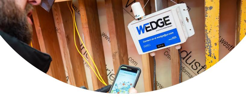
The WEDGE sensors were programmed to send alerts if the temperature rose above a certain threshold. Both United Rentals and the customer were able to monitor the real-time temperature data via the WEDGE dashboard.
